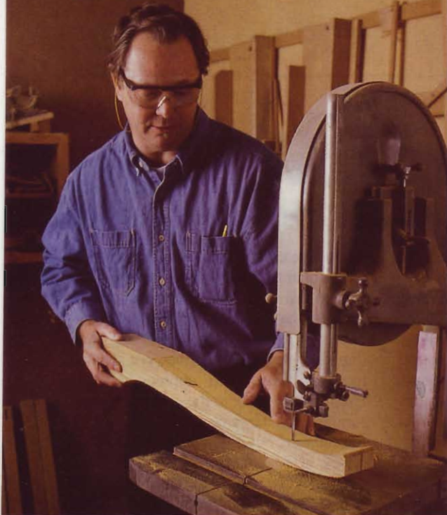
Greg freehands cypress through the bandsaw to rough out a cabriole leg.
